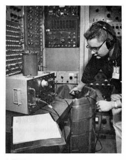
A TRANSDUCER is being used by James P. Quint, Northwestern co-op student, to check out operation of an underwater recovery unit in a test water tank.
